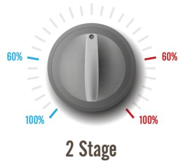
Better home heating and cooling systems have two stages, which make it a bit easier to control your home climate. Low stage is typically 50-70% of full capacity.
